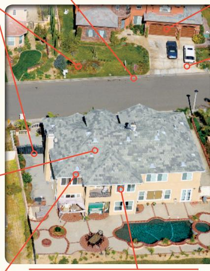
**Windows:** Heat from a wildfire can cause windows to break even before the home ignites. This allows burning embers to enter and start internal fires. Single-paned and large windows are particularly vulnerable.
